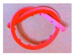
without losing its **flexible quality.** You just screw on the curved rail on the edge of given line and mill the contour on the **guiding ring** with a **router** or a **spindle moulder**.
