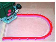
spindle moulder, the **hands are in a safe distance** behind the curved rail. On one-sided visible parts **"kurvenlinfix"** is screwed directly onto the workpiece for instance wall side pieces for staircases.
